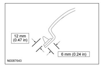
11. WARNING: Do not drive vehicle until the urethane adhesive seal has cured. Follow urethane adhesive manufacturer's curing directions. Inadequate or incorrect curing of the urethane adhesive seal will adversely affect glass retention. Failure to follow these instructions may result in serious injury to vehicle occupant(s).
